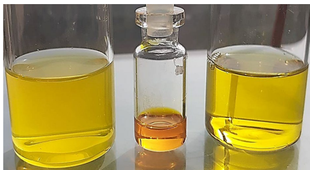
Fig. 1 Appearance of the water-based N. sativa essential oil nanoemulsions (after 48 h equilibration at 25 °C). Vials from left: nanoemulsion (F2), middle: pure unformulated essential oil, right: nanoemulsion (F1)
