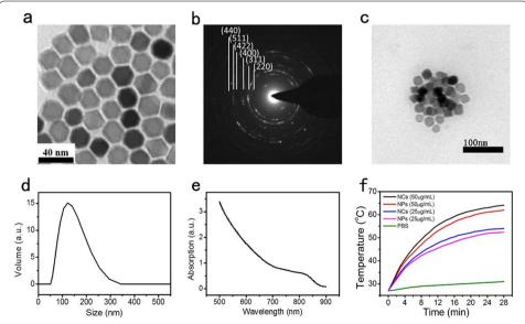
**Fig. 1** a TEM image of monodisperse  $Zn_{0.3}Fe_{2.7}O_4$  NPs, with an average diameter of 18 nm. **b** Electron diffraction showed typical cubic spinel structure. **c** Typical TEM image of  $Zn_{0.3}Fe_{2.7}O_4$  nanoclusters; **d** size distribution of  $Zn_{0.3}Fe_{2.7}O_4$  nanoclusters tested by dynamic light scattering. **e** Absorption spectra of  $Zn_{0.3}Fe_{2.7}O_4$  nanoclusters. **f** Heating curves of different concentrations of NPs or NCs upon 808-nm laser irradiation.
