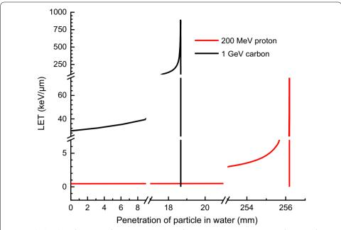
**Fig. 2** Calculated LET for proton of 200 MeV and carbon of 1 GeV propagating in water as a function of penetration from SRIM code (Wishart and Rao 2010; Ziegler et al. 2010). Plots exhibit peaks of LET, namely Bragg peak, corresponding to the last slowdown of the particle in liquid water. These plots do not account for nuclear processes like fragmentation
