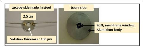
**Fig. 8** Pictures presenting both sides of the flow-cell used in fluorescence microscopy. 200 nm  $Si_3N_4$  membrane is provided from SPI Supplies
