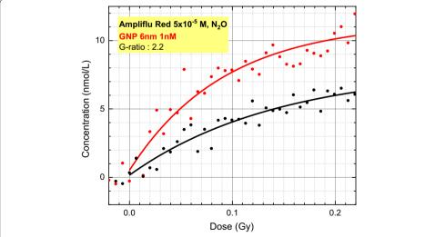
**Fig. 5** Concentration of Resorufin formed under α-rays as a function of dose delivered to solution. In black, without GNP; in red, with GNP of 6 nm at concentration of 1 nM. Dose rate was deduced, considering an empirical exponential growth of the Resorufin.  $N_2$ O saturated solution of Ampliflu® Red was used at a concentration of  $5 \times 10^{-5}$  M in phosphate buffer. The initial rate shows a ratio of 2.2 between the slopes in solutions in presence and in absence of GNP
