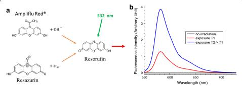
**Fig. 7** Resorufin formation processes from oxidation by hydroxyl radical using Ampliflu<sup>®</sup> Red molecule and from reduction by hydrated electron using resazurin (**a**). 532 nm light exposure of irradiated solution leads to the fluorescence of Resorufin with a spectral spanning which is shown in **b**, given after radiation exposure times of 0, T1 and T2 > T1 (T is not defined here. It serves only for demonstration. T depends on the dose rate provided by radiation)
