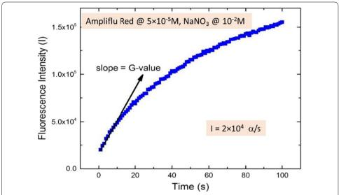
**Fig. 9** Fluorescence intensity calibrated with Resorufin solutions was obtained by the intensity integration of each image recorded every second (exposure time of 20 ms). This curve was obtained by using Ampliflu<sup>®</sup> Red at concentration of  $5 \times 10^{-5}$  M and sodium nitrate at  $10^{-2}$  M aiming to scavenge hydrated electron. Beam intensity was roughly  $2 \times 10^4$  α-particles per second
