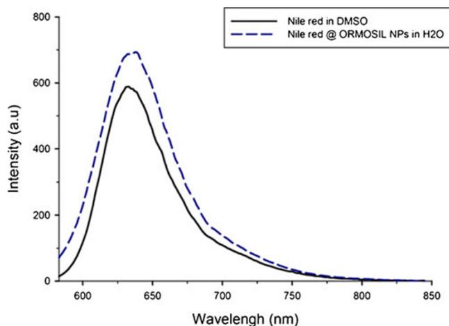
**Fig. 5** Fluorescent spectrum of Nile Red dissolved in DMSO and Nile Red encapsulated in ORMOSIL nanoparticles
