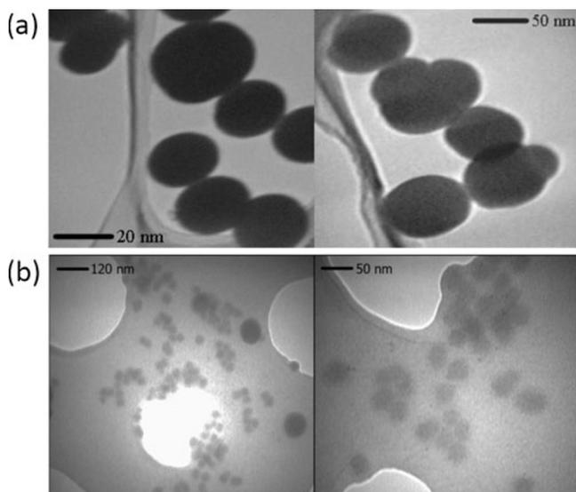
**Fig. 2** TEM images of ORMOSIL nanoparticles synthesized using AOT (AOTORM NPs) (a), and ORMOSIL nanoparticles synthesized using Tween 80 (TWORM NPs) (b)
