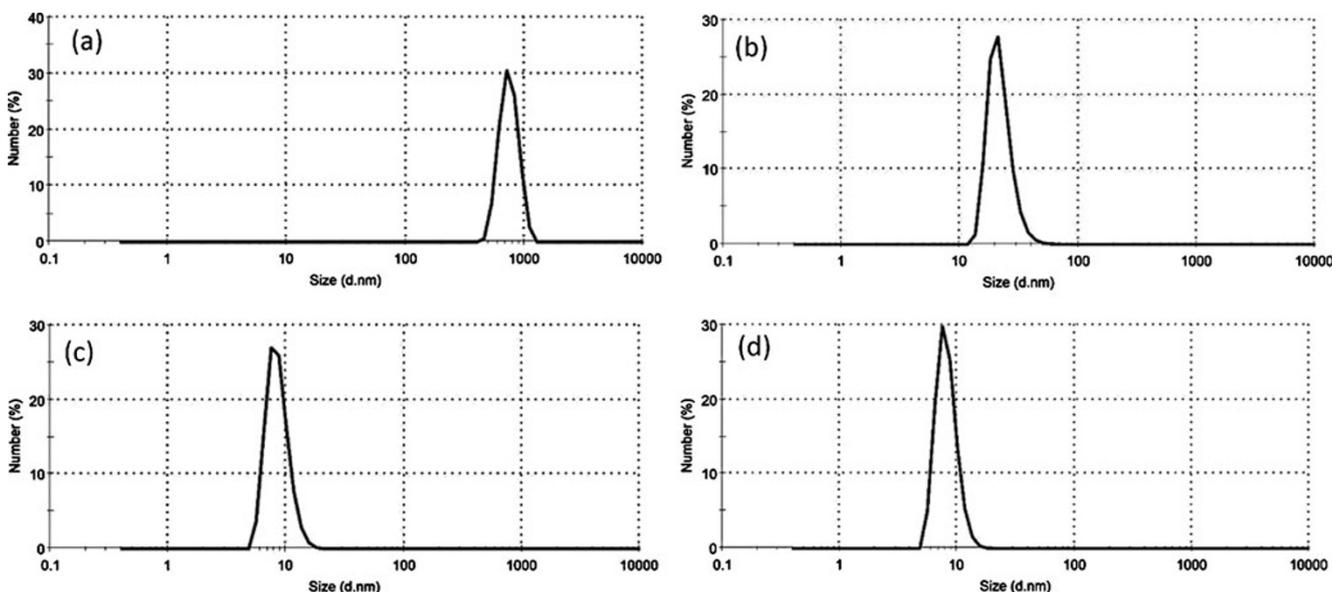
**Fig. 3** Average hydrodynamic size distribution obtained by DLS from AOT micelles (a), AOTORM nanoparticles (b), Tween 80 micelles (c), and TWORM nanoparticles (d) with the mean size of 749, 35, 11.7, and 10.9 nm, respectively
